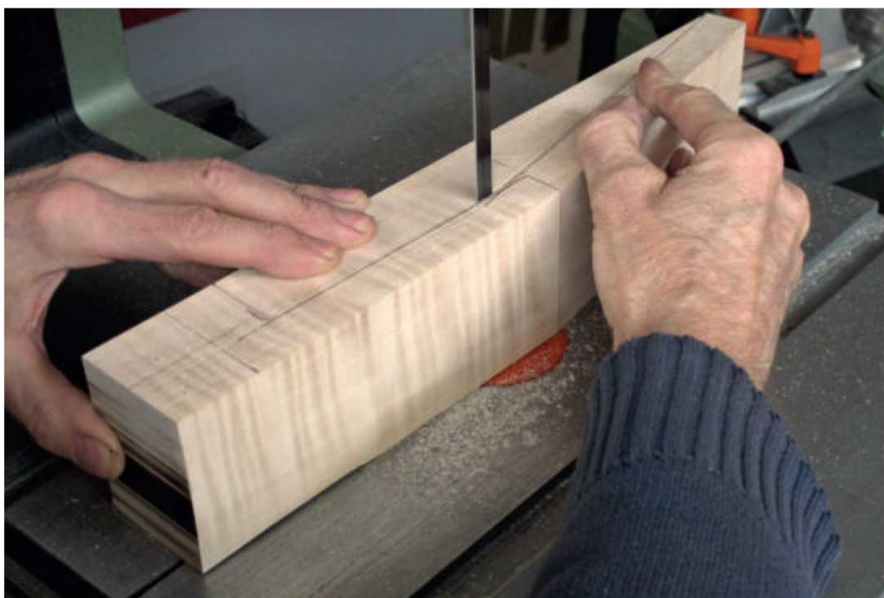
Fig. 10-3. Sawing out the neck blank on a band saw
